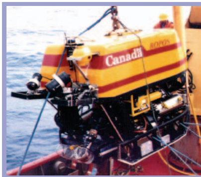
ISE's ROPOS - a 5000 meter depth ROV built in 1985 for science and research
